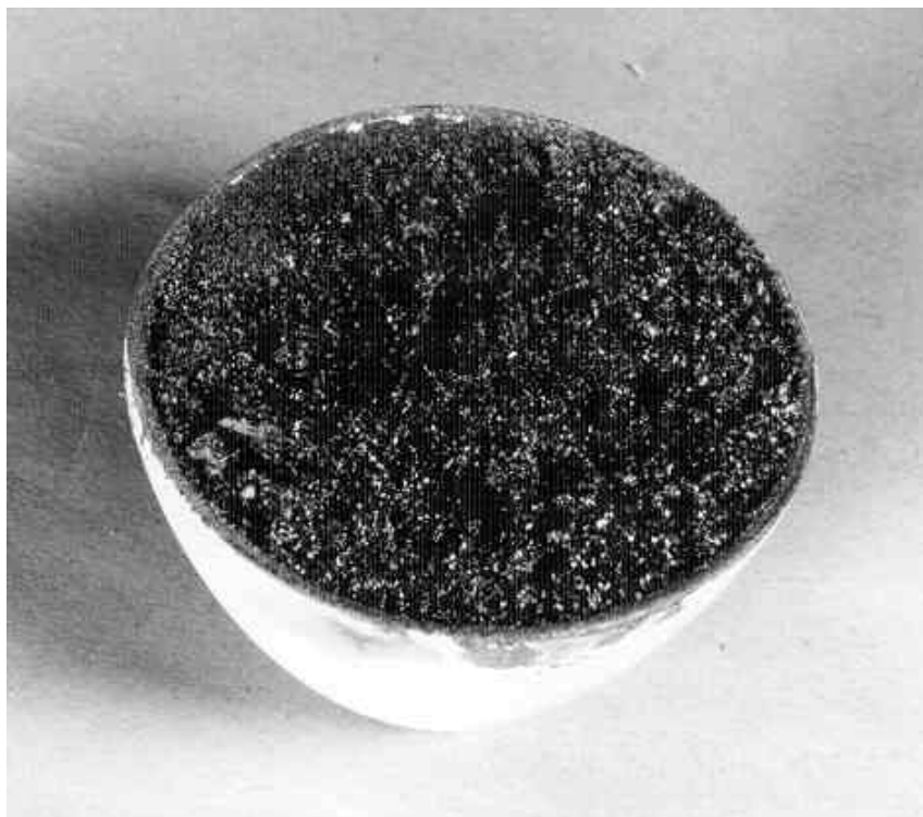
Figure 1. Proteinoid material created by spraying a solution of amino acids onto a hot crucible in a furnace.
